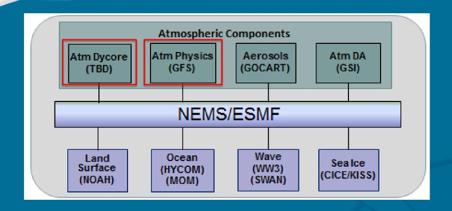
Modular modeling, using ESMF to modularize elements in fully coupled unified global model
