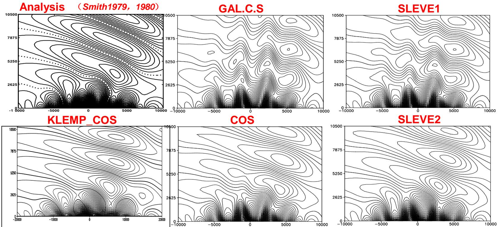
mountain wave: Cross-section of vertical velocity  $W$  after 10 hours integration
