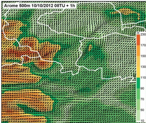
500m simulation in Paris area to provide wind and turbulence related parameters to a wake-vortex prediction model (here wind field over surface orography)
