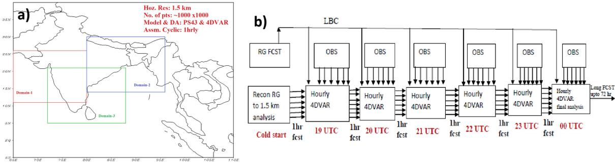
Fig-1: a) Configured different domains for HRRR DA over Indian region and b) Schematic diagram of 1hrly HRRR DA cycle.
