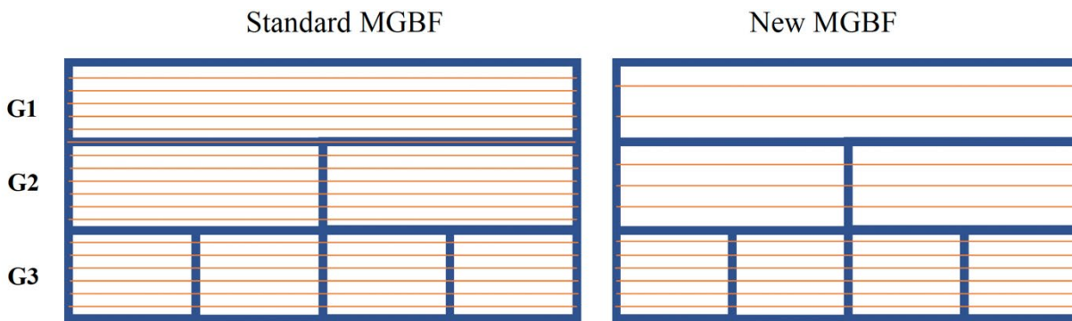
Fig. 1. On the left, schematically presented standard MGBF paradigm, in which vertical resolutions of all grid generations are treated equally. On the right, the latest MGBF version, in which vertical resolutions of successive grid generations are systematically reduced (halved). The thick grid boxes represent processors; G1, G2, and G3 denote successive grid generations 1, 2 and 3.
