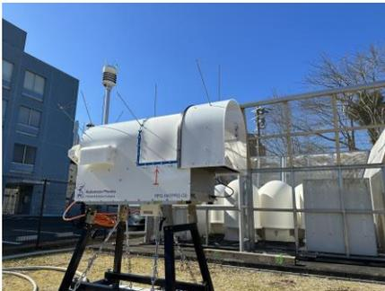
Figure 1. Overview of MWR station at Owase. The equipment in the foreground is MWR and the one in the background is WPR.
