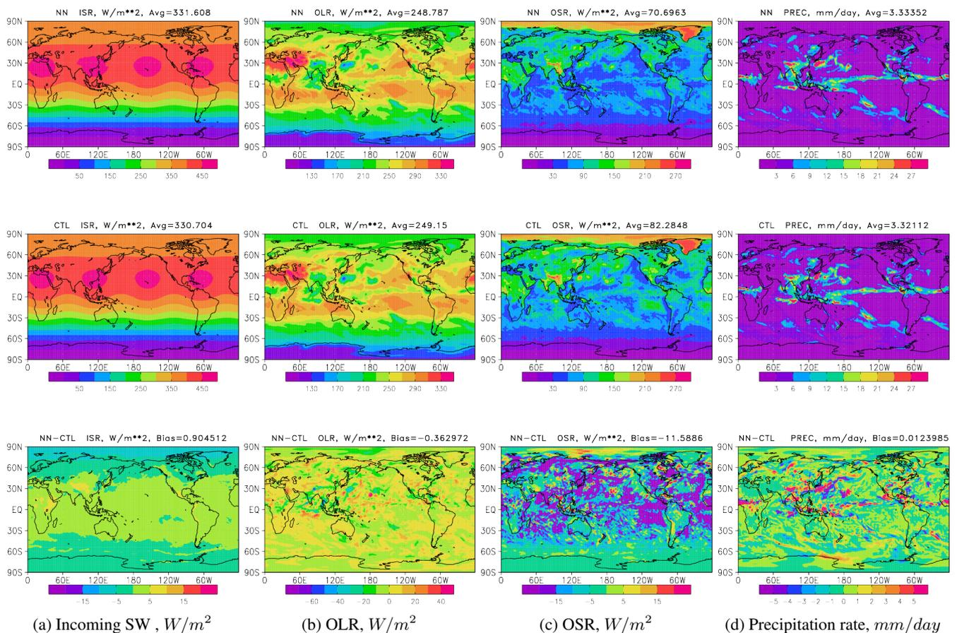
Figure 1: Full NN radiation vs control, Zhao-Carr MP, day 3-10 average of a C96 forecast initialized at 00Z on 8/1/17.
