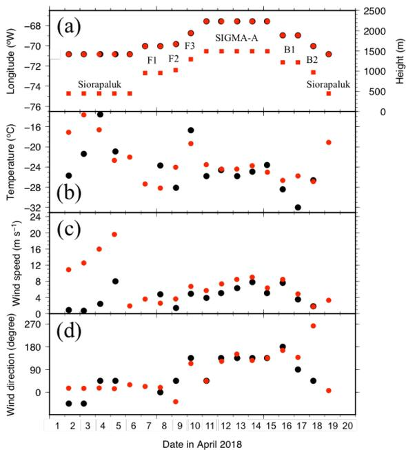
Fig. 3. Observed (black) and simulated (red) weather elements at the campsite every morning. (a) Longitude (circles) and height (squares), (b) air temperature, (c) wind speed, and (d) wind direction.
