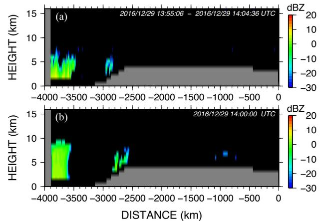
Fig. 5 Cloud reflectivity (a) observed by CloudSat Cloud Profiling Radar on 29 December 2016 along the orbit shown in Fig. 1 and (b) simulated by Joint Simulator from output from the JMA-NHM.
