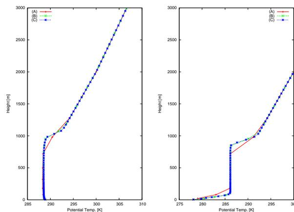
Fig. 1: Vertical profiles of potential temperature in the GABLS2 experiments. Left: when the mixed layer is fully developed; right: when the stable layer is evolved. Each line corresponds to grid configurations (A), (B) and (C) shown in Table 1.
