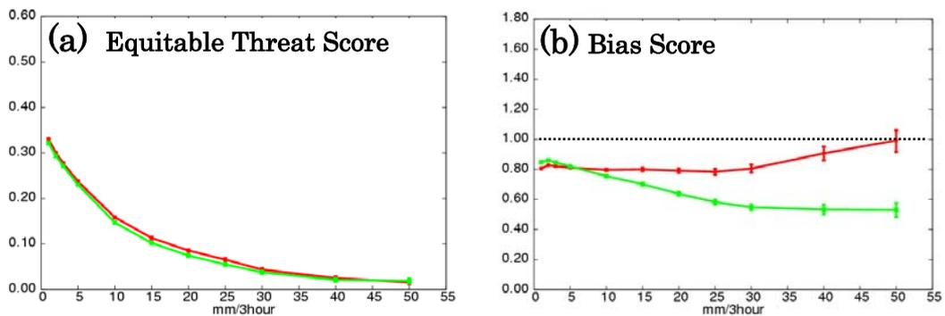
Fig. 2 Statistical verification results for three-hourly accumulated precipitation of MSM forecasts against radar-raingauge analyzed precipitation based on the contingency table in the term between 7<sup>th</sup> and 26<sup>th</sup> July, 2009: (a) equitable threat score; (b) bias score. The scores for MSM forecasts using the modified KF scheme are indicated by the red line, while the original ones are indicated by the green line, with error bars showing a 95% confidence interval.
