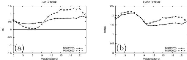
Fig. 2: Verification of surface temperature for each valid time. (a) Time sequence of ME in summer. (b) Same as (a), but of RMSE.
