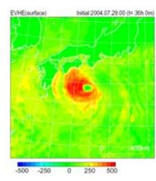
Figure 10 Latent heat flux by the coupled model at T+36h.
