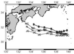
Figure.7 JMA best track positions (B), the predicted positions of hydrostatic coupled model (JC), nonhydrostatic model (N), and nonhydrostatic coupled model (NC).
