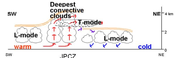
Fig. 2: Schematic structures of cloud bands associated with JPCZ observed on 14 January 2001 (from Murakami et al., 2002).
