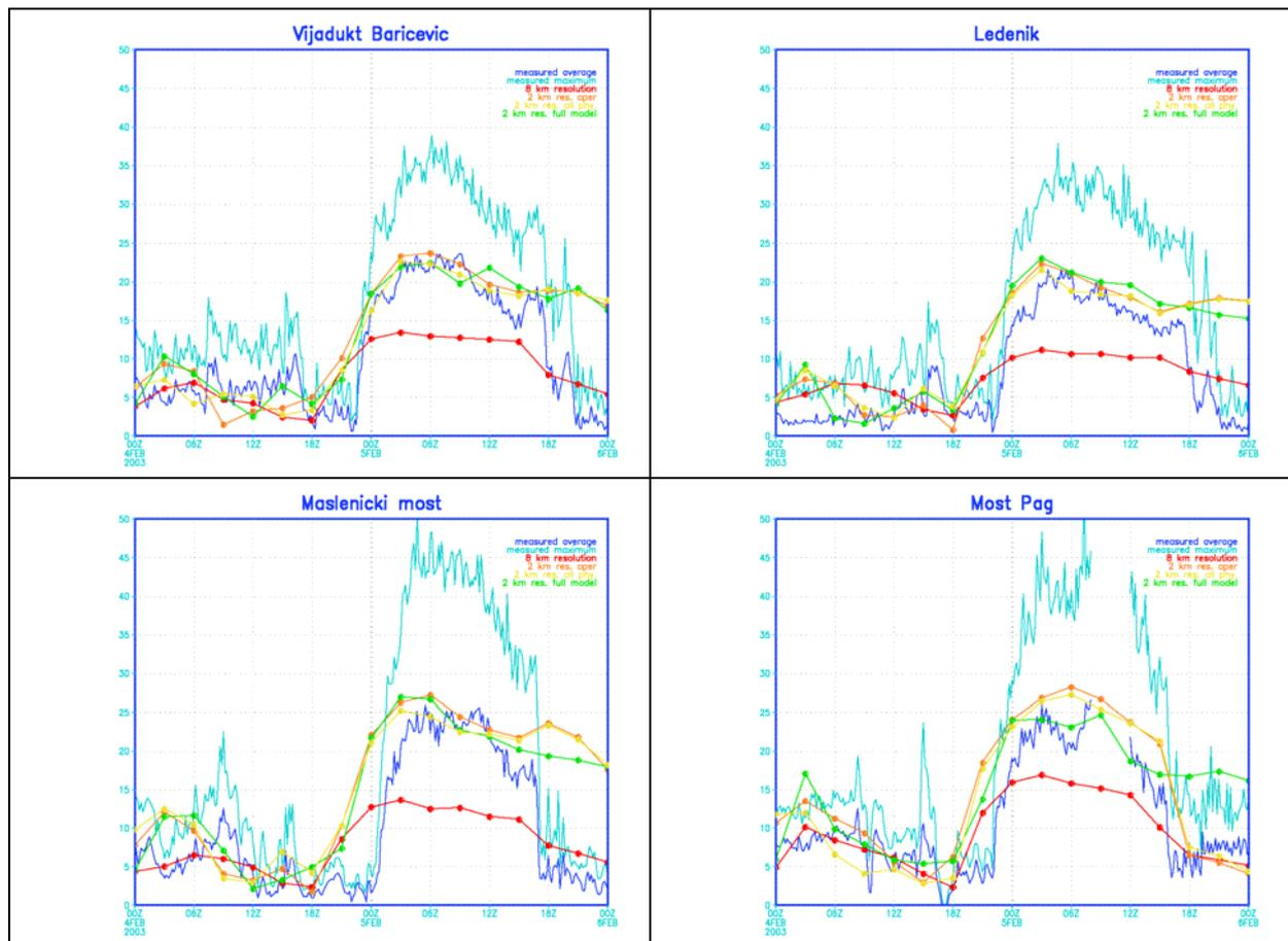
Figure 2. Measured wind speed from automatic stations and modeled data for the 00 UTC run on February 4<sup>th</sup> 2003 from the closest model point. Measured 10 min average wind speed in m/s (dark blue), 10 min maximum (light blue), 8-km resolution model forecast (red), 2-km resolution dynamical adaptations; operational (orange), using whole physics package (yellow) and 2-km resolution 48-hour model integration (green).
