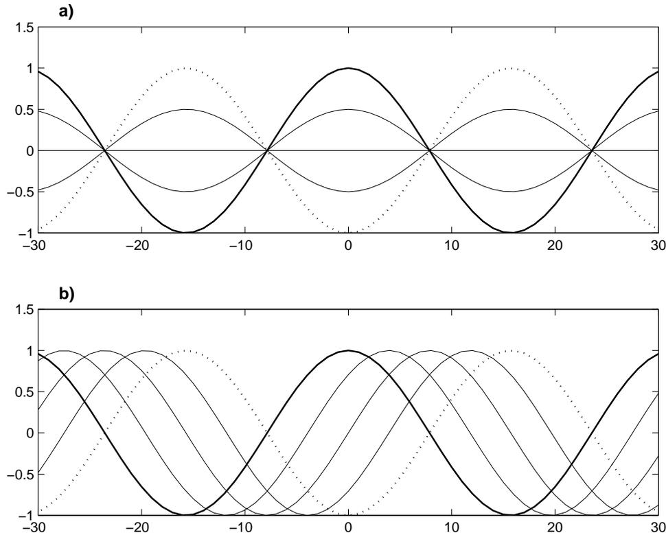
**Figure 2.** Position of the feature between two sampled times interpolated by a) weighted linear interpolation and b) the complex empirical orthogonal function interpolation method. The thick and dotted lines represent the position of the wave at time  $t = 0$  and  $t = 1$  respectively, and the thin lines represent the estimated positions at times  $t = 1/4$ ,  $t = 1/2$ , and  $t = 3/4$ .
